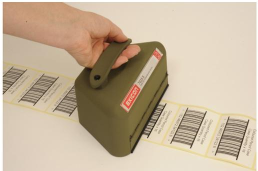
The verifier should be placed either just above or just below the barcode and the trigger pressed. With the trigger still pressed, move the verifier down the height of the barcode. The verifier will scan at the rate of 100 verifications a second until it reaches the bottom of the barcode (or gets to the maximum number of scans).
